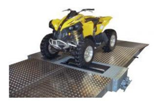
• Full motorcycle testlanes available with wheel clamp and powered speedometer tester.
